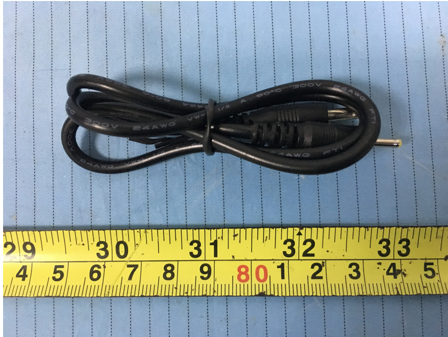
EUT – DC Power Cable View
