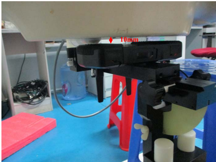
Test Position_Back Antenna Fold (10mm)
