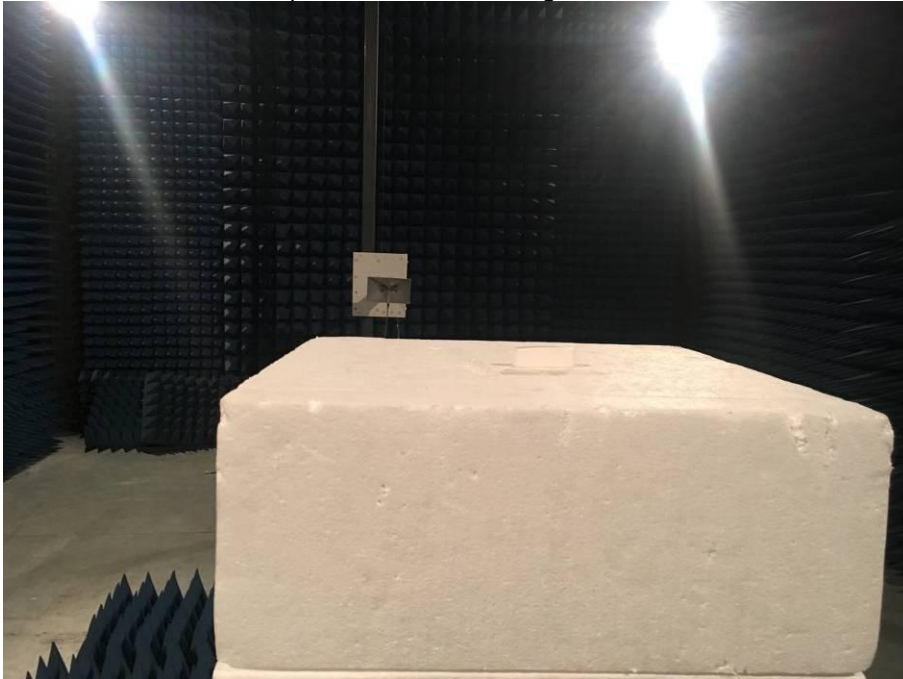
Above 1GHz: Test height 1.5m, the styrofoam block placed in the 0.8 m high test table
