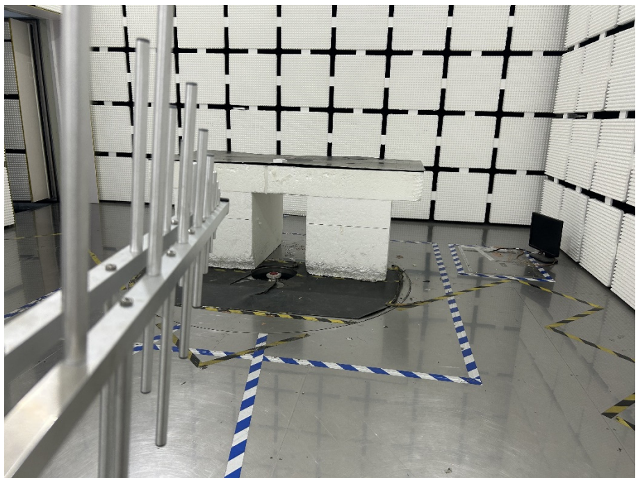
Radiation Emission Test Setup (30MHz to 1GHz)
