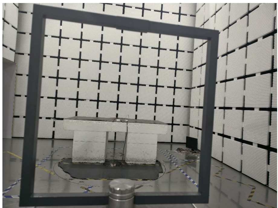
Radiation Emission Test Setup (Below 30MHz)
