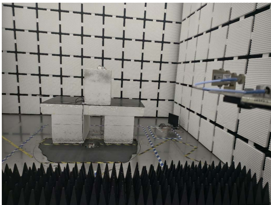
Radiation Emission Test Setup (Above 18GHz)
