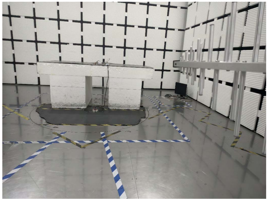
Radiation Emission Test Setup (30MHz to 1GHz)
