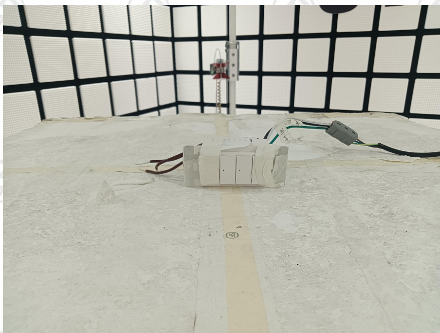
Radiated spurious emission Test Setup-2 (Above 1GHz)
