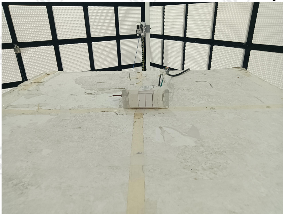
Radiated spurious emission Test Setup-3 (Above 18GHz)
