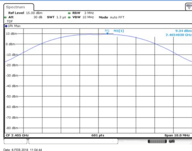
O-QPSK LOW CHANNEL
