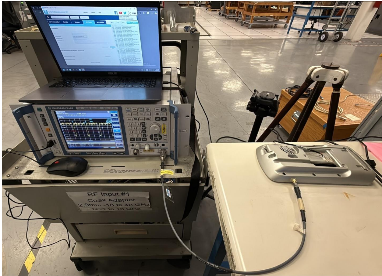
Conducted Emissions at Antenna Port
