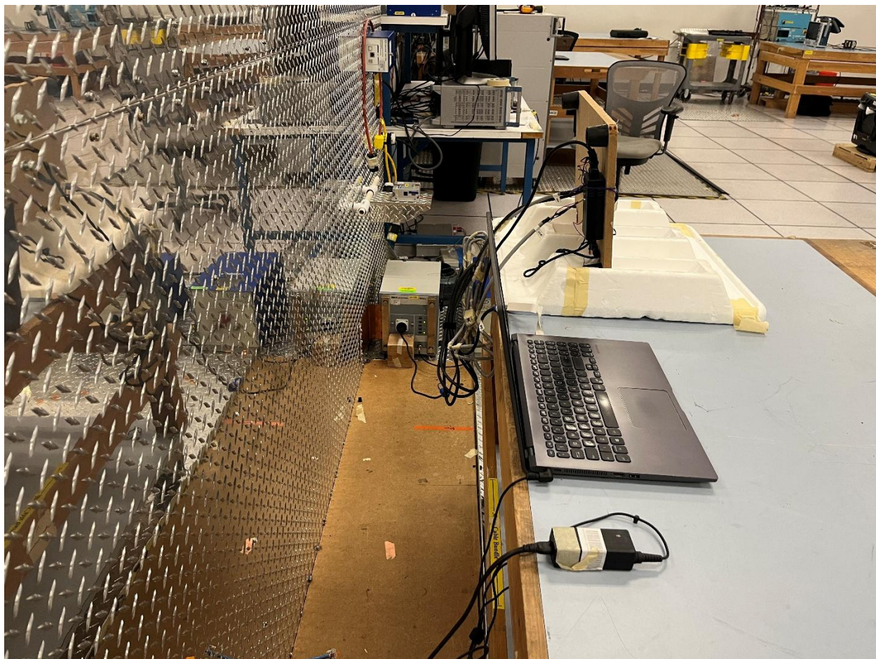
Conducted Emissions at AC Mains (Side View)
