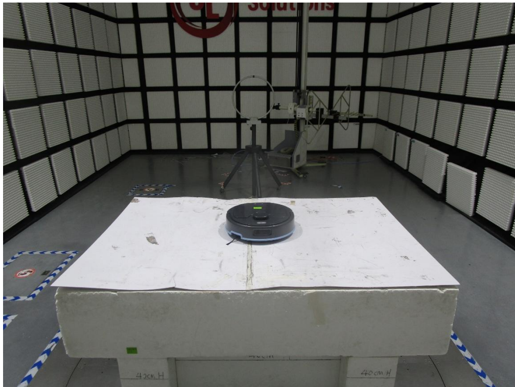
RADIATED RF MEASUREMENT SETUP (Below 30MHz)
