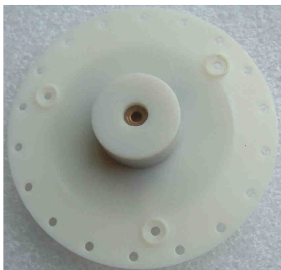
Static part of turbine
