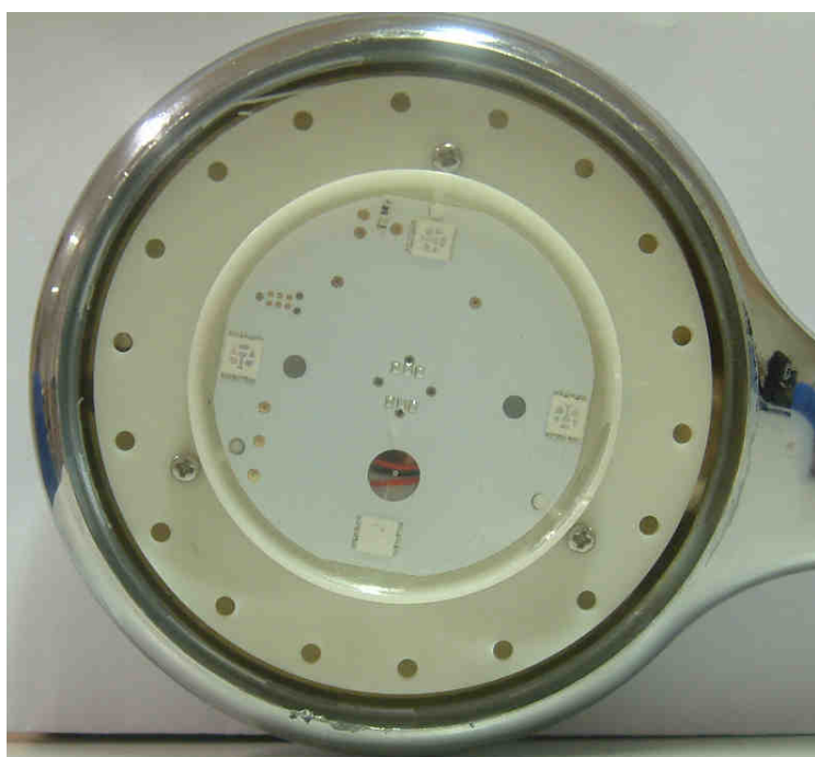
PCB view (inside translucent resin)
