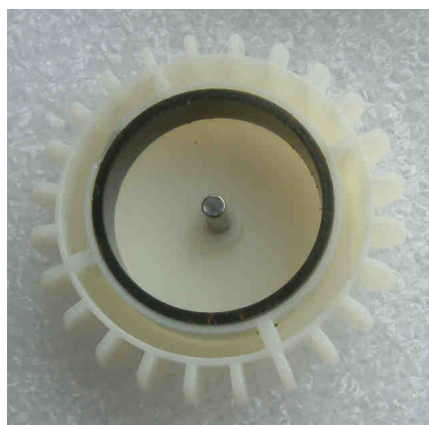
Magnet inside turbine
