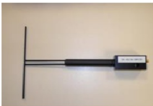
Figure 1 – Satimo COMOSAR Validation Dipole
