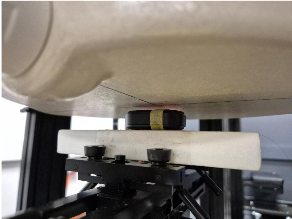
Figure A SAR Test Setup – Body – Back Side 5mm
