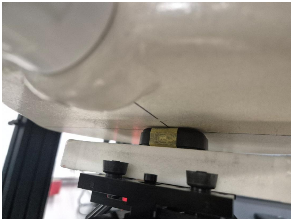
Figure B SAR Test Setup – Extremity – Front Side 0mm
