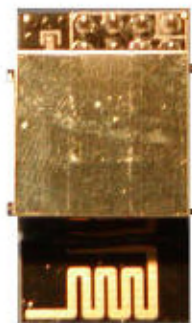
RF Module NRF24WDS rev A Top Side with RF shield
