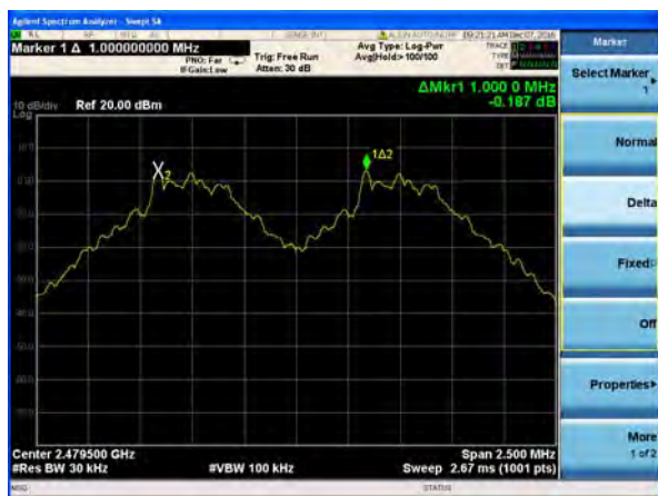
(1Mbps) Channel Separation plot on channel 77-78
