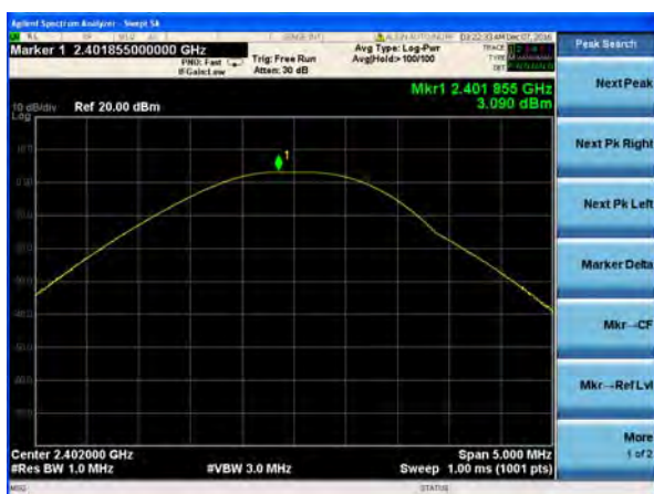
Peak output Power plot on channel 39 (1Mbps)
