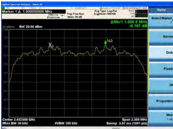
(2Mbps) Channel Separation plot on channel 39-40
