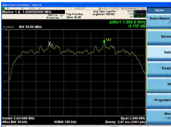
(2Mbps) Channel Separation plot on channel 39-40
