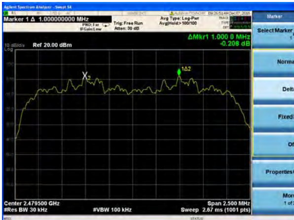
(2Mbps) Channel Separation plot on channel 77-78
