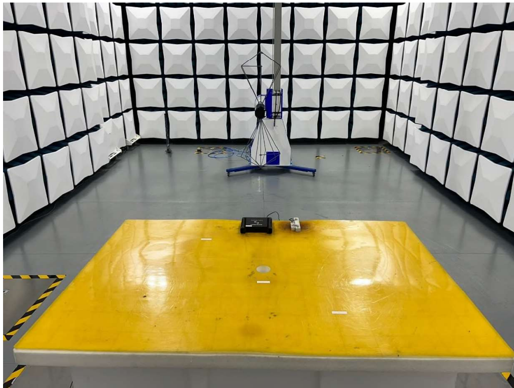
Set up for Radiated Emission 30M~200MHz (PoE supply)
