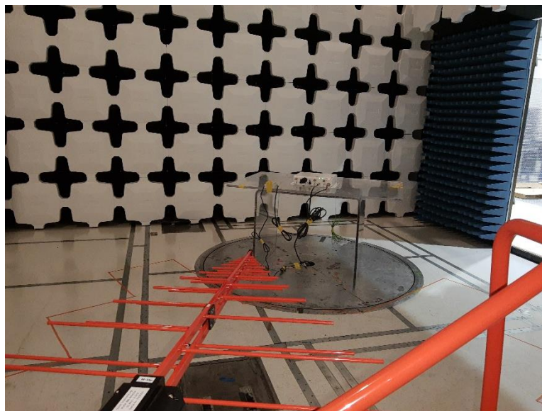
Figure 62. REE Test Setup below 1GHz
