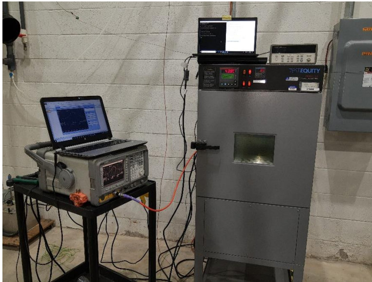
Figure 64. Frequency Stability Test Setup
