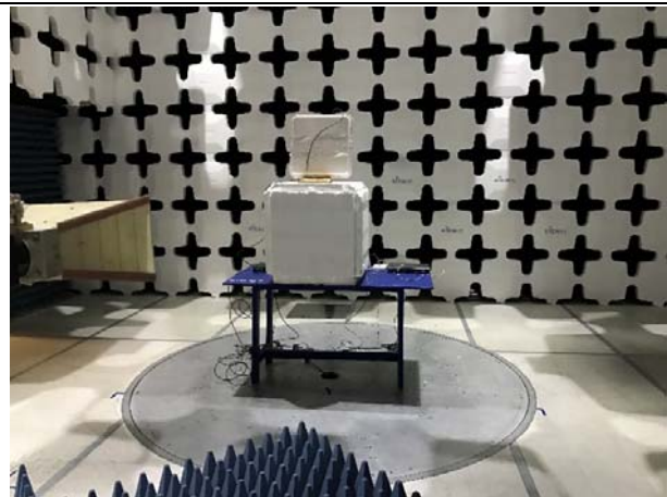
Radiated Emissions (>1GHz) – Rear View
