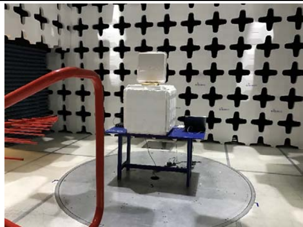
Radiated Emissions (<1GHz) – Rear View
