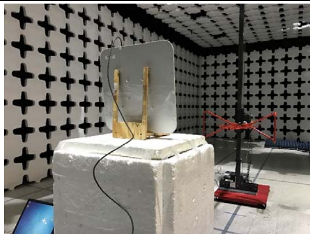
Radiated Emissions (<1GHz) – Front View
