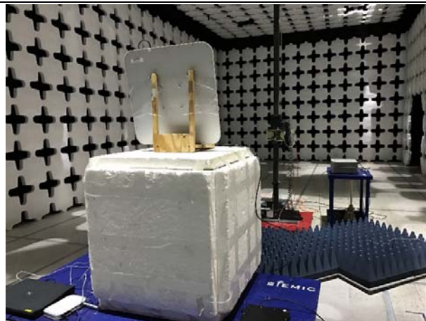
Radiated Emissions (>1GHz) – Front View
