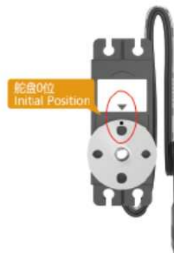
连接正确后，舵机会转动至0位 Disc is back to initial position
