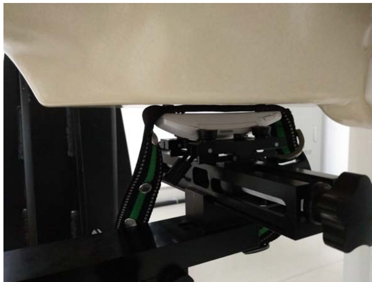
Limb-worn SAR Setup Photo
