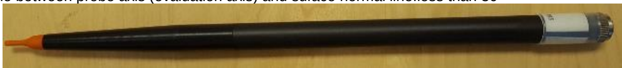
Figure 2 – MVG COMOSAR Dosimetric E field Dipole
