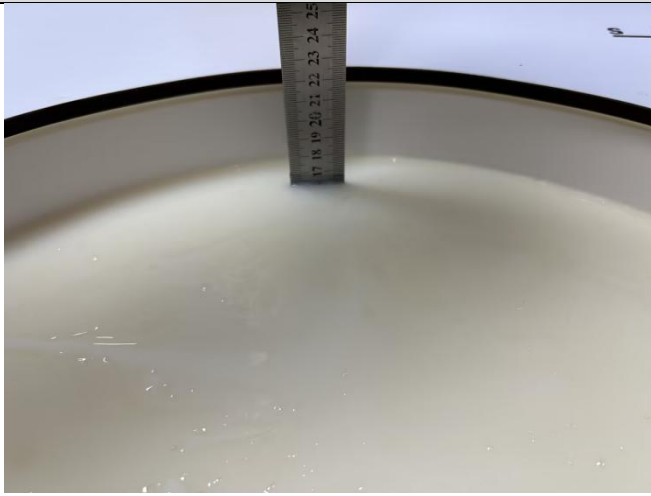
Photo 1: Tissue Simulant Liquid for Head 700-3000MHz
