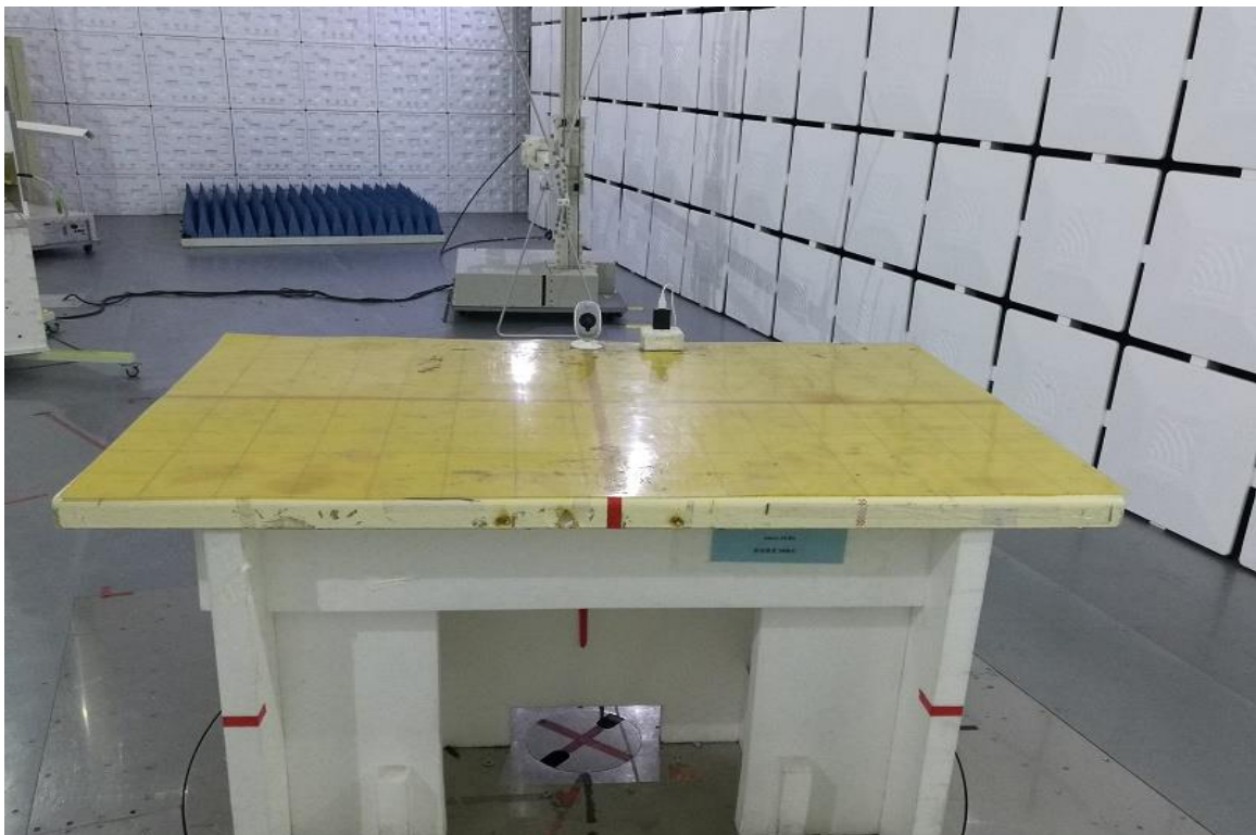
Photograph 6: Set-up for Radiated Emissions, below 1GHz
