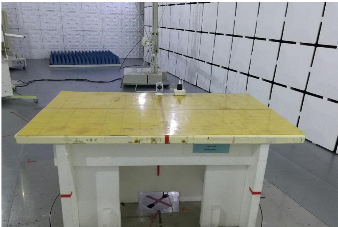
Photograph 6: Set-up for Radiated Emissions, above 1GHz
