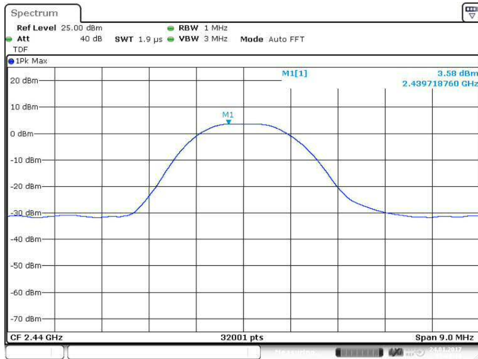
Figure 2: Conducted power (ch mid)
