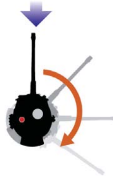
Fig. 11b Pull the Right Joystick , the tank turret can be proportionally controlled to rotate right.
