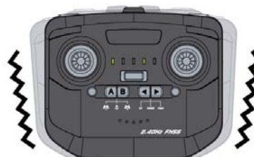
Fig. 5.2a When the Power Switch is right to the "POWER" position, the vibration function is enabled.
