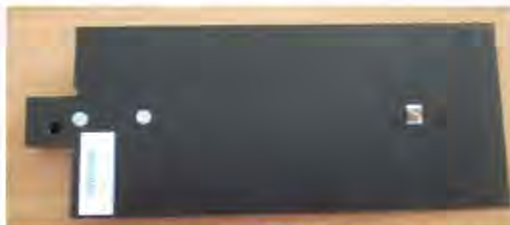
Figure 1 – MVG COMOHAC Validation Dipole
