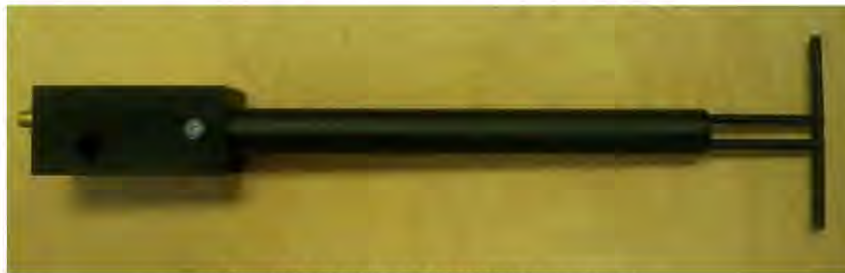
Figure 1 – MVG COMOSAR Validation Dipole
