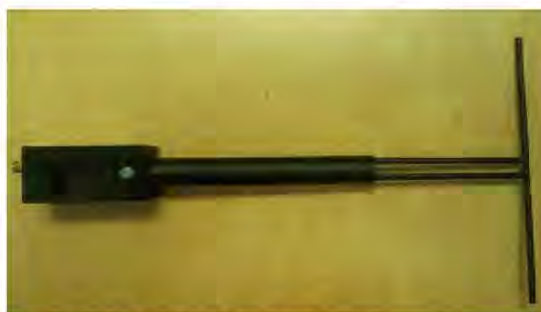
Figure 1 – MVG COMOSAR Validation Dipole
