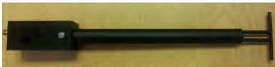
Figure 1 – MVG COMOSAR Validation Dipole
