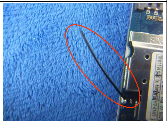
BT - Antenna View
