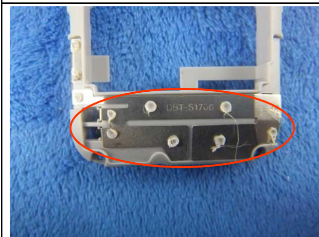
GSM/PCS Antenna View
