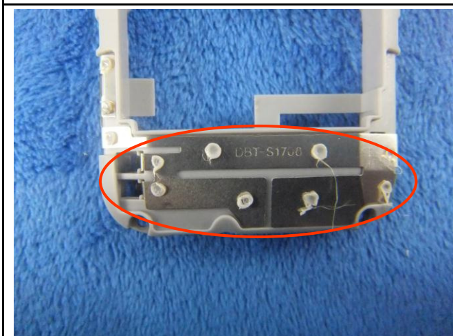
GSM/PCS Antenna View
