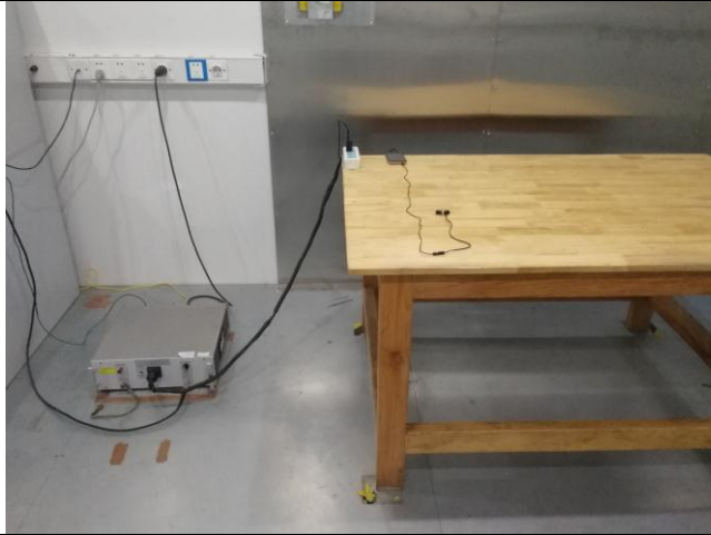
Conducted Emissions Test Setup Front View
