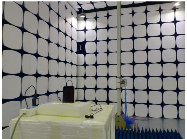
Radiated Spurious Emissions Test Setup Above 1GHz
