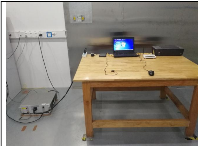
Conducted Emissions Test Setup – Front View
