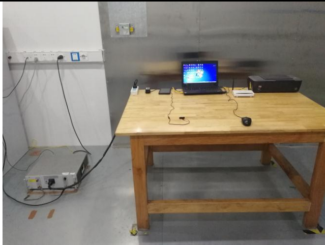
Conducted Emissions Test Setup – Front View
