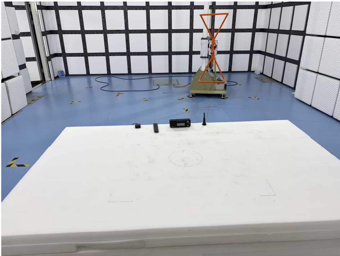
Radiation Emission - Back View (Below 1GHz)
