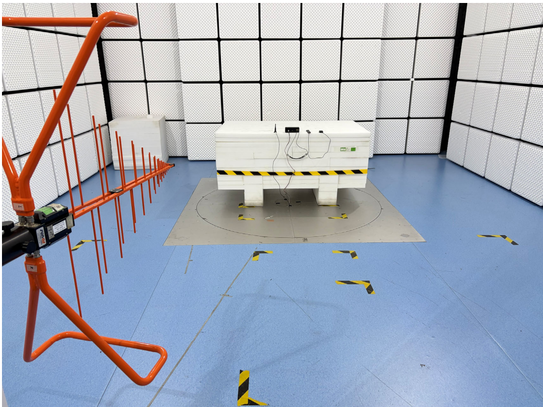
Radiation Emission - Back View (Below 1GHz)
