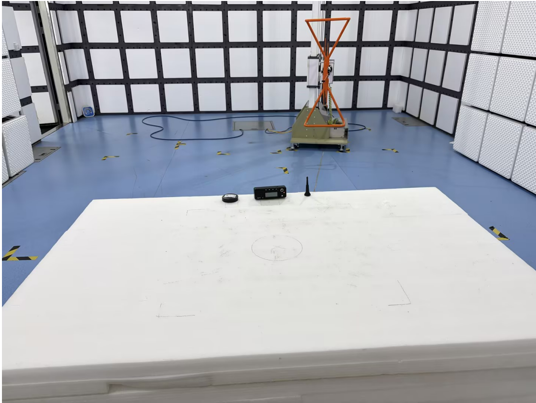
Radiation Emission - Back View (Below 1GHz)
