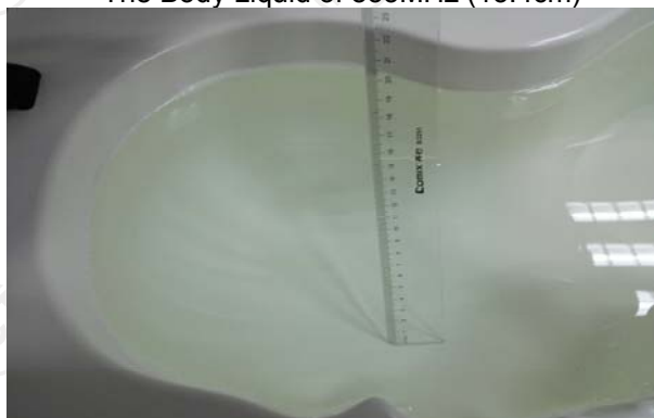
The Head Liquid of 1900MHz (15.5cm)
