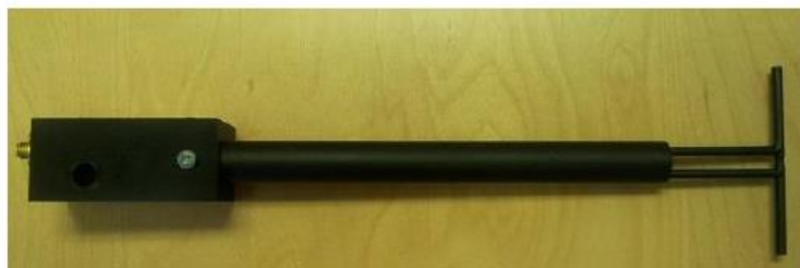
Figure 1 – MVG COMOSAR Validation Dipole
