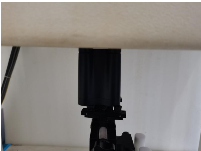
Fig-4.3 Bottom of EUT with 0 cm Gap (Body Mode)
