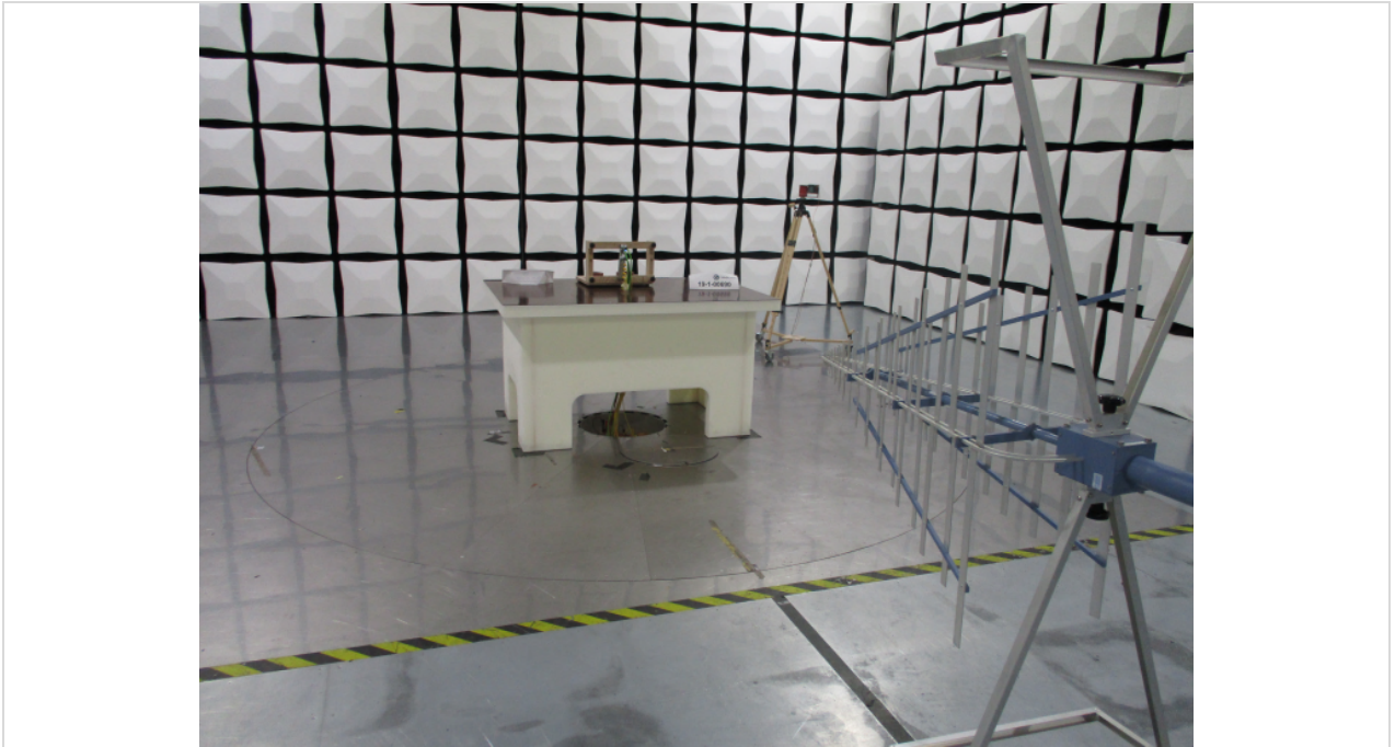
Photograph 1: Radiated emission measurements test set-up for measurement of frequency up to 1000 MHz Preliminary measurement in 3 m test distance
