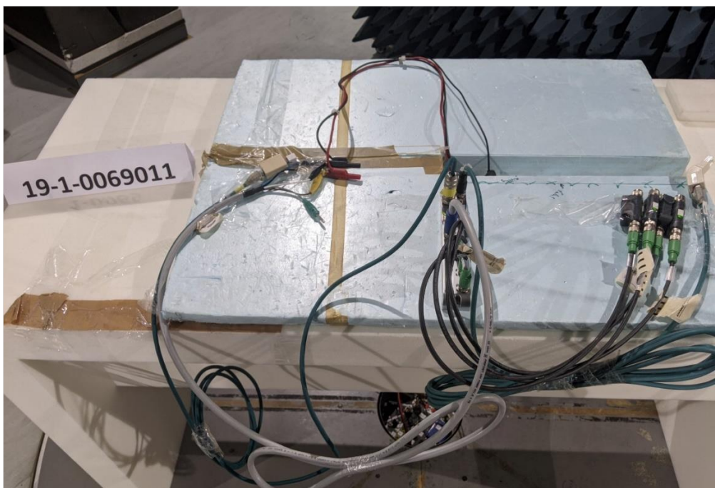
Photograph 4: EUT Setup Magnetic Field Measurements in the Semi anechoic chamber
