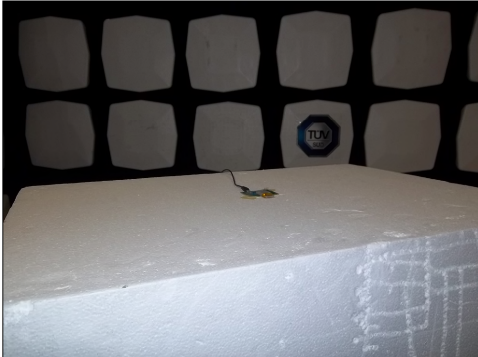
Figure 5: Equipment Under Test – Radiated Emissions Z-orientation
