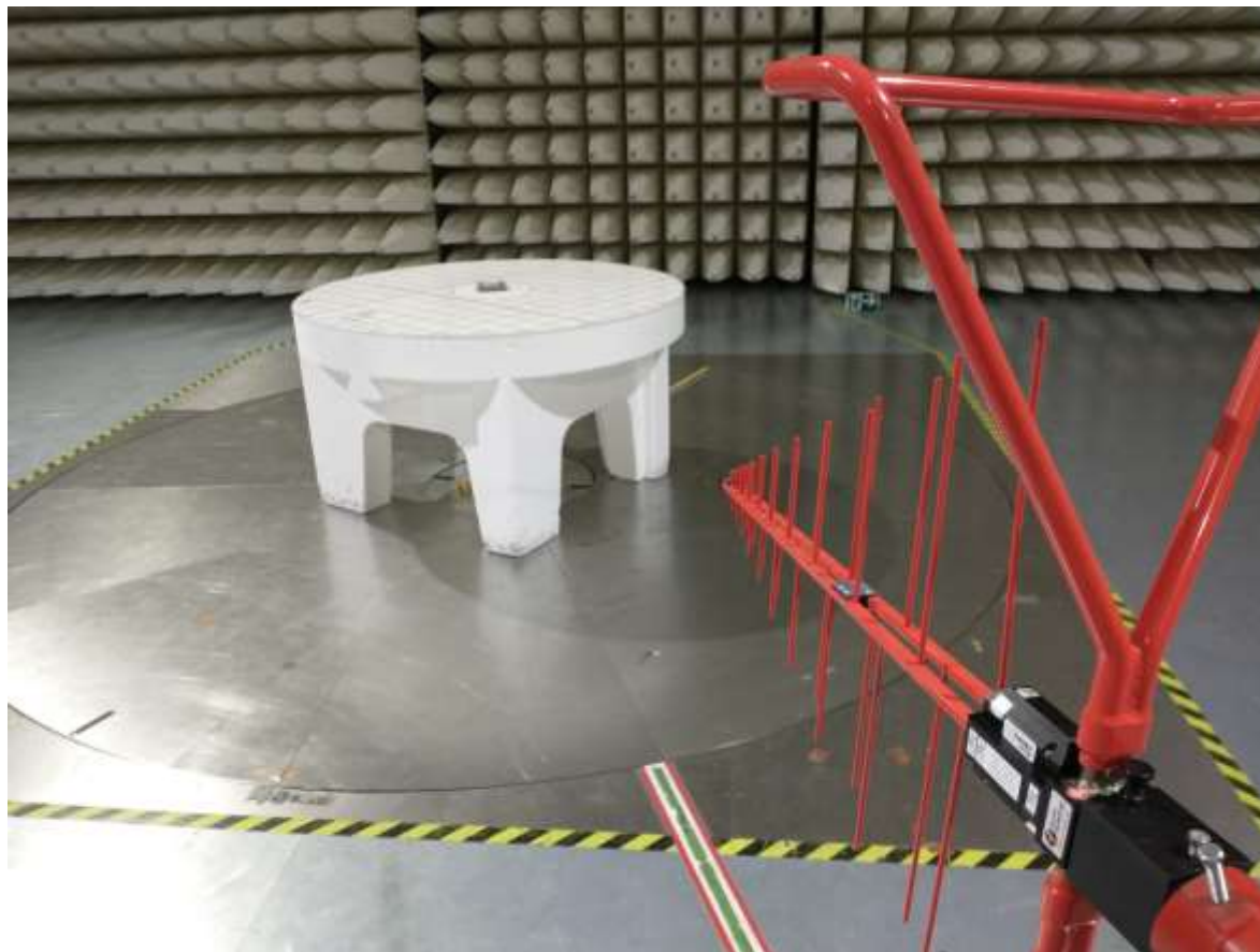
Figure 27. 30-1000MHz Radiated Test Setup
