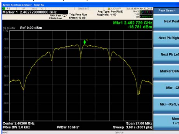
(802.11b) PSD plot on channel 11
