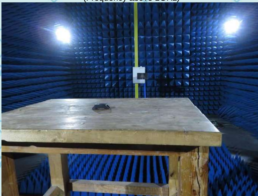
RADIATED EMISSION TEST (Frequency above 1GHz)
