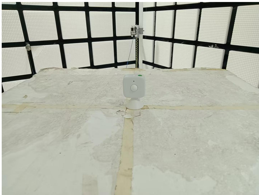
Radiated spurious emission Test Setup-3(18GHz-41GHz)
