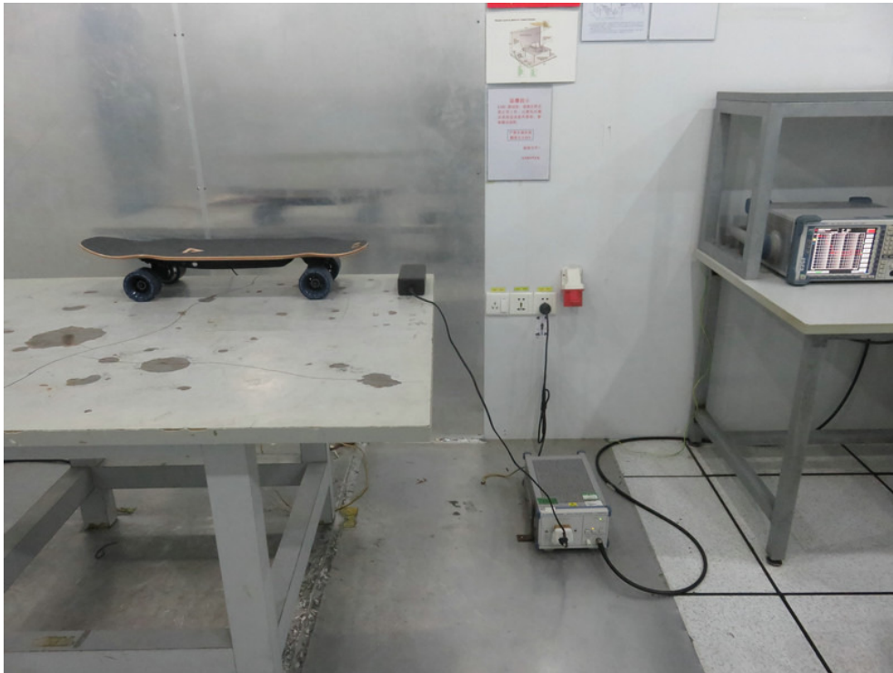
Photo of Conducted Emission Measurement
