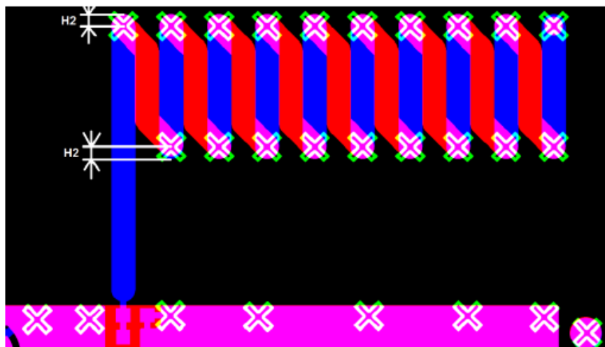
Figure 3. Zoom of Top and Bottom Layer Layout with Via Markings
