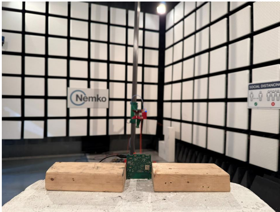
Figure 7.1-10: Radiated Spurious emissions setup photo – above 1 GHz
