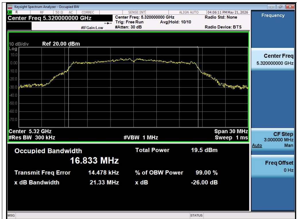
Test_Graph_802.11a_Chain A_5320_6Mbps_OBW
