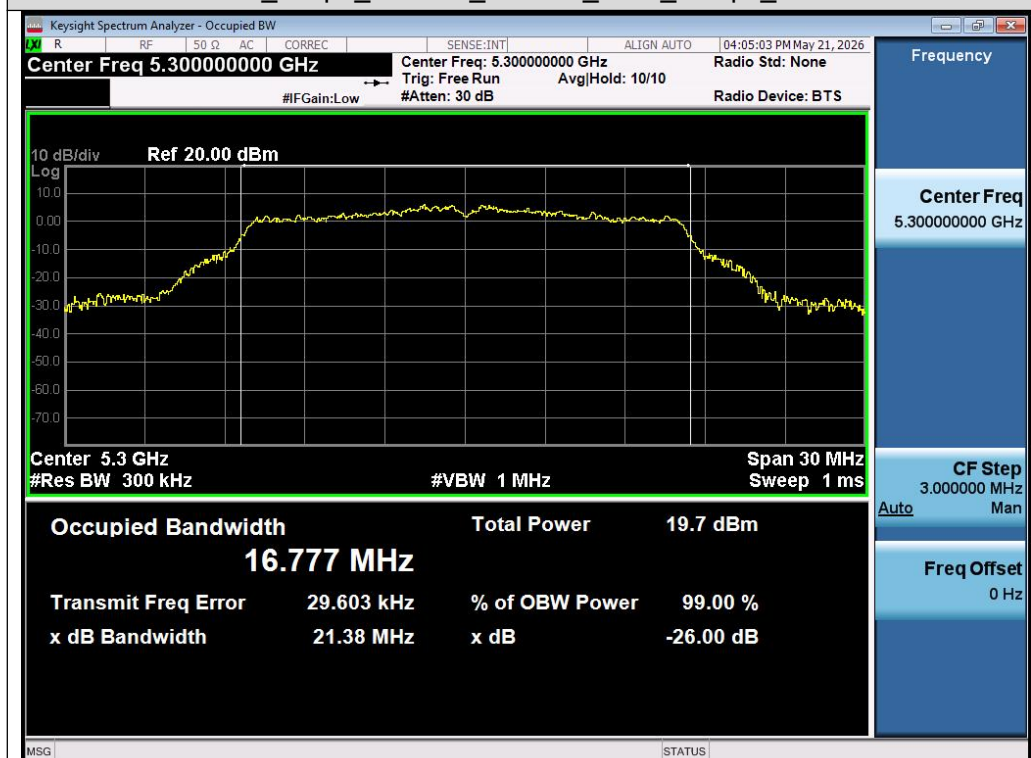
Test_Graph_802.11a_Chain A_5300_6Mbps_OBW
