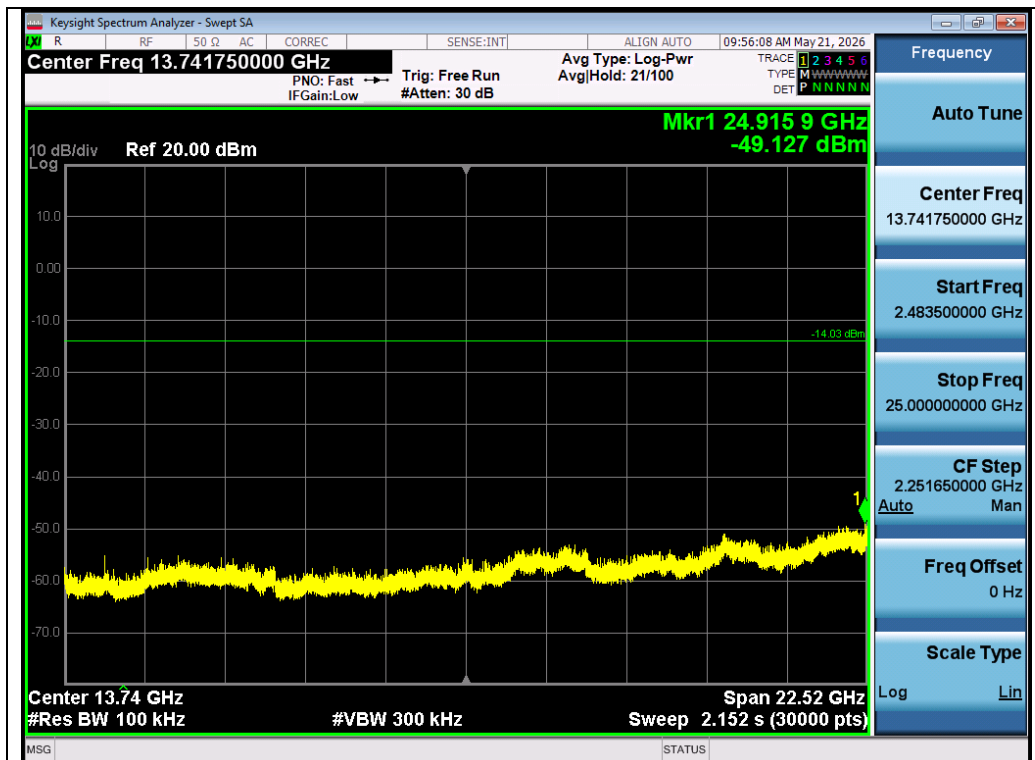
Test_Graph_802.11b_Chain A_2412_1Mbps_Lower Band Edge Emissions
