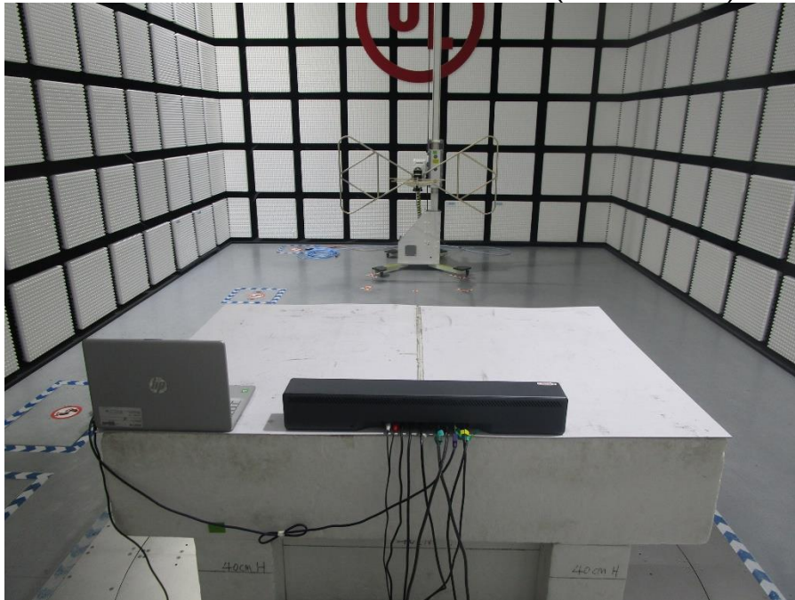
RADIATED RF MEASUREMENT SETUP (Below 30MHz)
