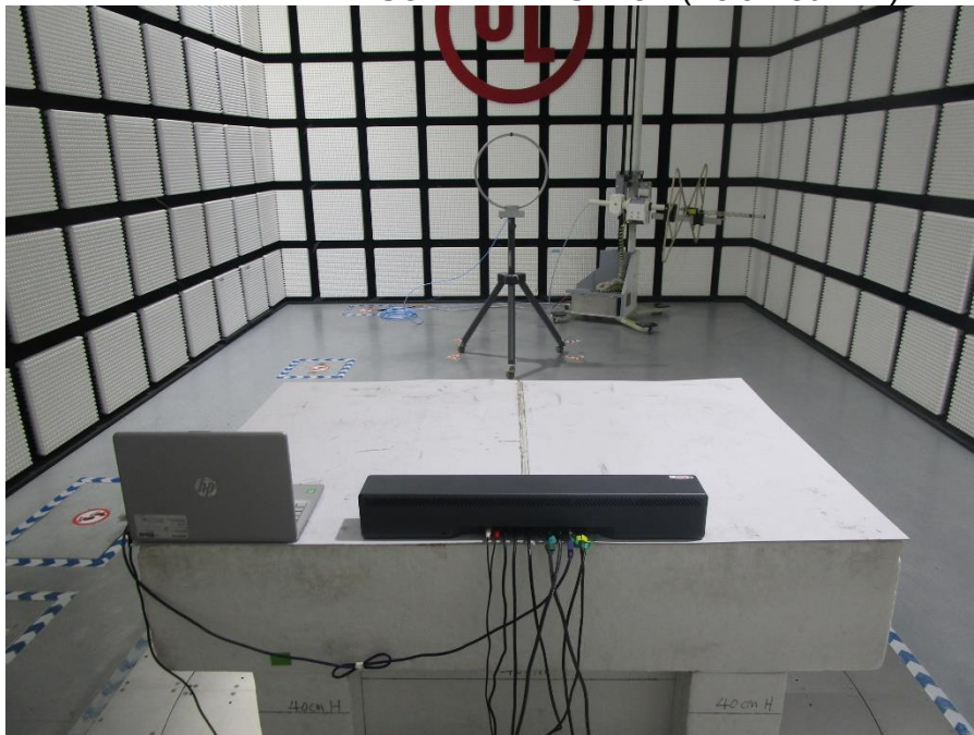
RADIATED RF MEASUREMENT SETUP (Below 30MHz)
