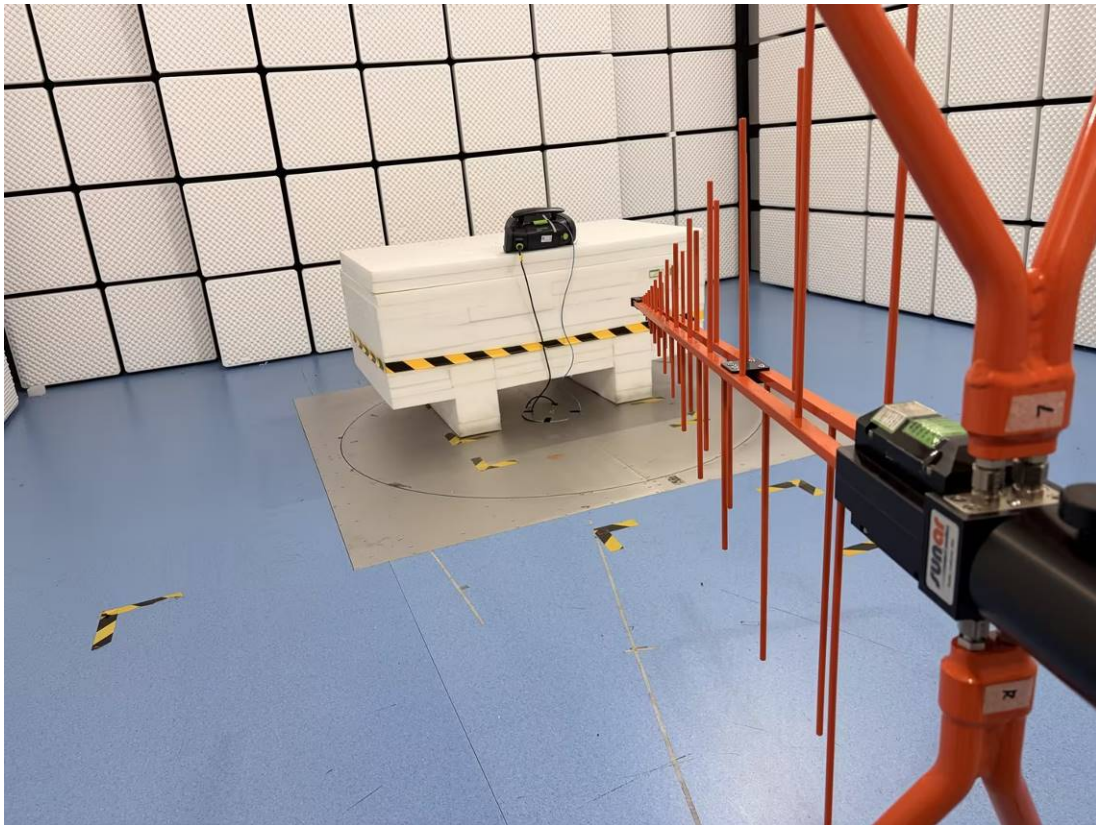
RE – Front View (30MHz~1GHz)_Powered by Battery(BP 18 Li 5,2 AS)
